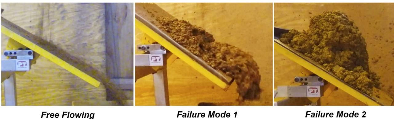
FIG 5 – Experimental impact testing modes of failure.
